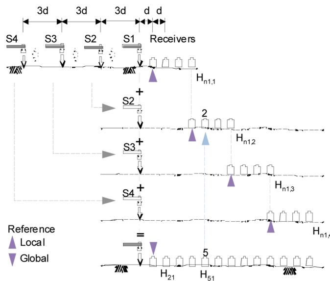
FIGURE 2. Schematic diagram to combine waveforms from a different set of source functions by the proposed walk-away testing method
