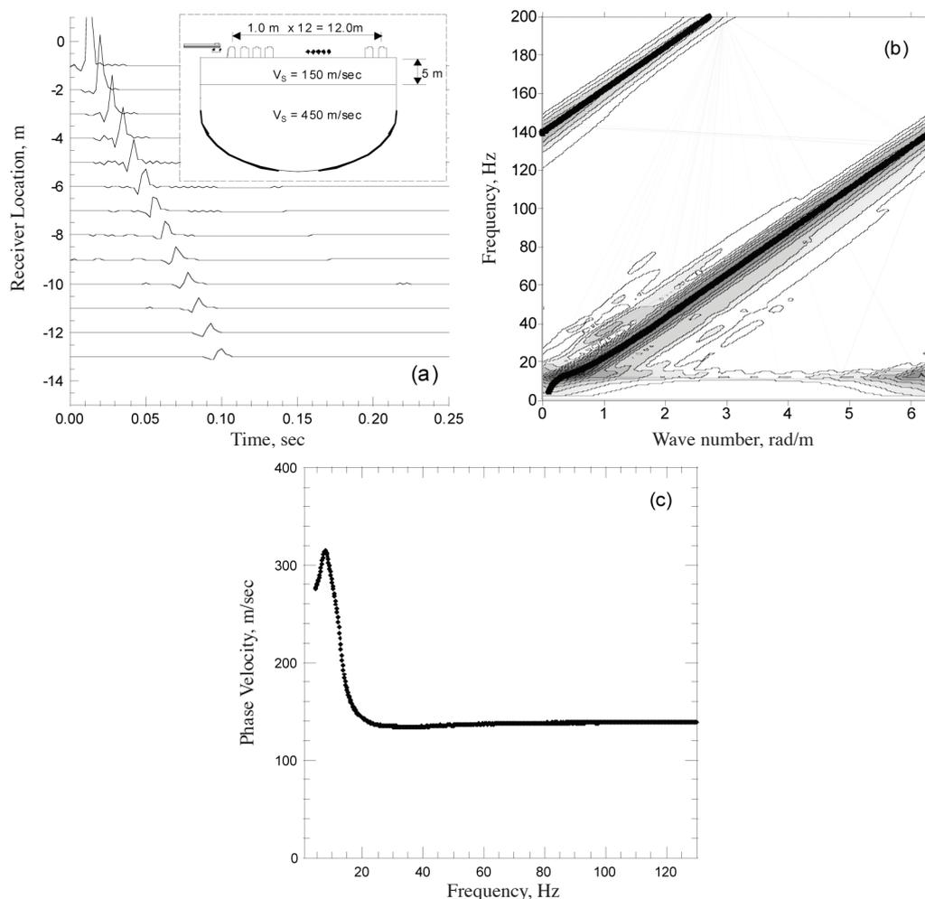
FIGURE 1. Application of beamforming technique to synthetic waveforms determined at a shallow bedrock site: (a) synthetic waveforms, (b) frequency-wavenumber map and (c) phase velocity dispersion curve
