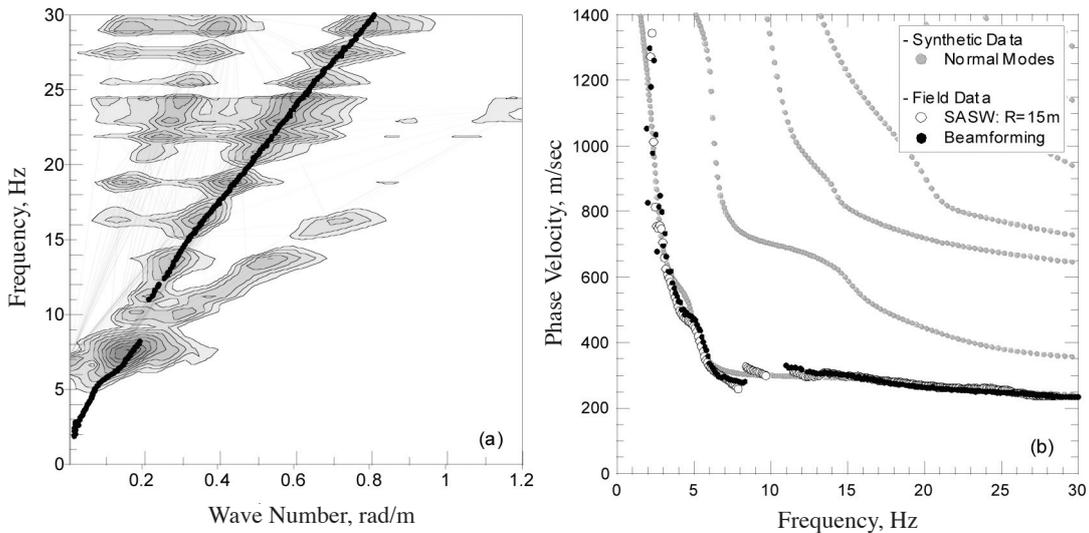
FIGURE 5. Results of beamforming tests at a natural geotechnical site near Hornsby, Texas: (a) f-k spectrum and (b) phase-velocity dispersion curve
