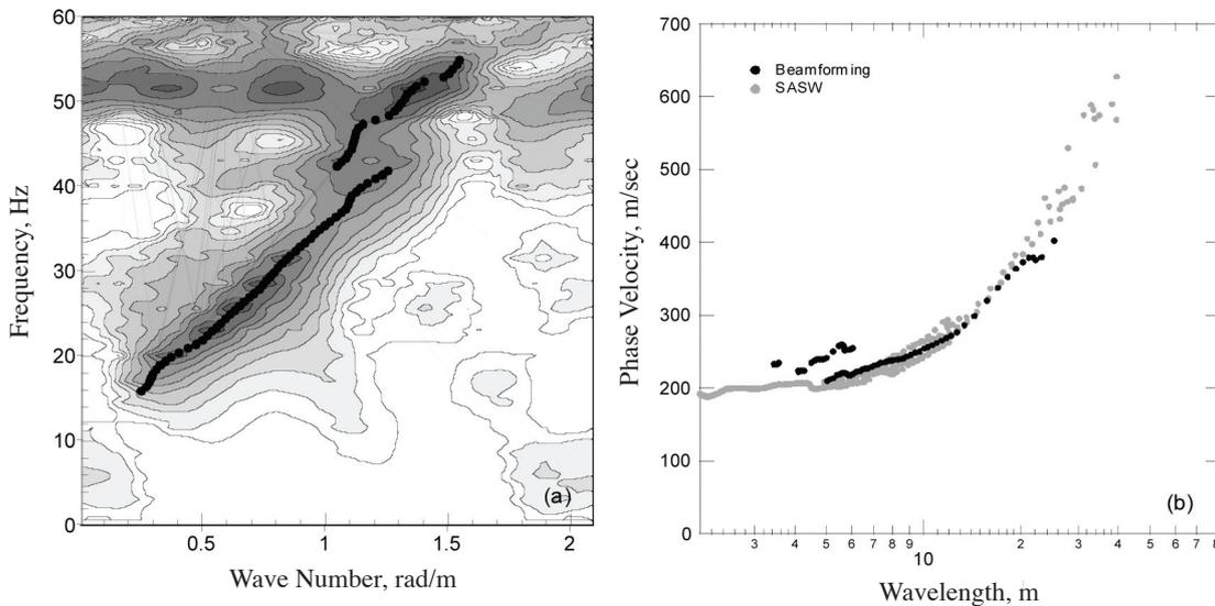
FIGURE 6. Results of beamforming tests at a natural geotechnical site in DaeGu, Korea: (a) f-k spectrum and (b) phase-velocity dispersion curve
