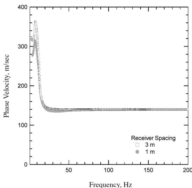
FIGURE 4. Resulting dispersion curves based on recovered wave numbers in Figure 3
